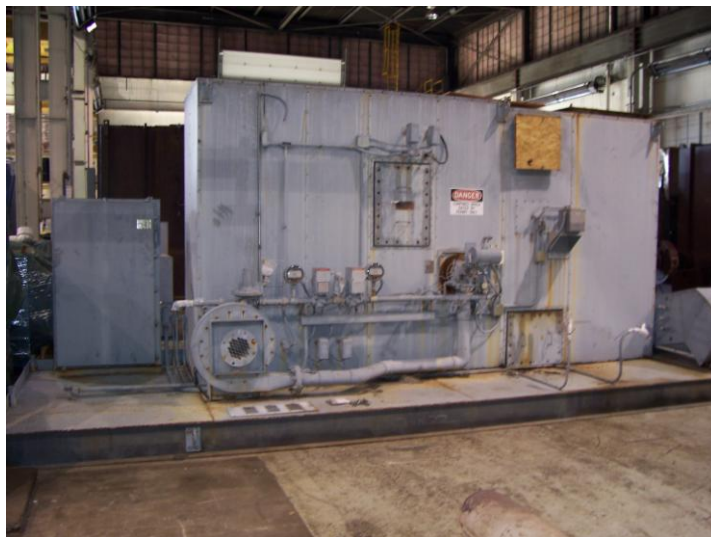
Figure 12: Catalytic Thermal Oxidiser
