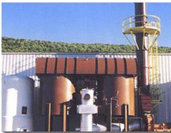
Figure 13: Schematic of Regenerative Thermal Oxidiser
