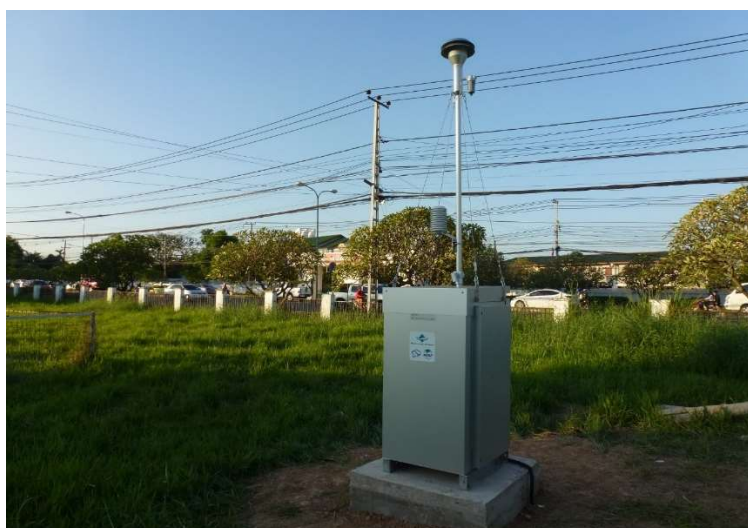
Figure 1.3. Ambient Air Quality Monitoring Station.
